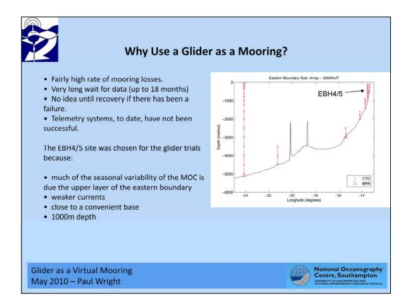
The RAPID array traverses the Atlantic at approximately 26N. The Western boundary is steep to, while the eastern boundary is more shelving. This has meant that the eastern sub-array needs to consist of a number of moorings.
