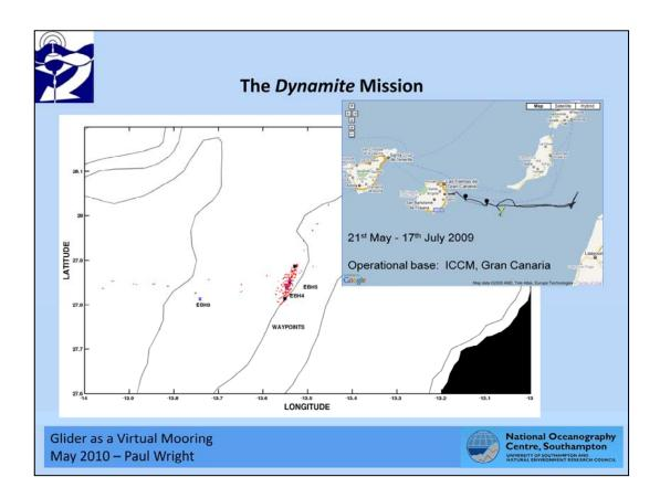
The chart above shows the inshore mooring locations and the GPS locations of the glider when she surfaced. The black stars are the waypoints used to constrain the glider around the EBH4/5 location. The glider rarely was > 4km from the moorings.
