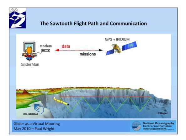
Due to the method of flying the glider describes a saw tooth like path. On surfacing the glider performs the following:
