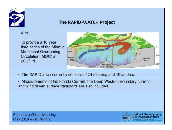
The RAPID array measures the Meridional Overturning Circulation (MOC), which is the net northward transport of the warmer upper level water from the equatorial region to the poles.
