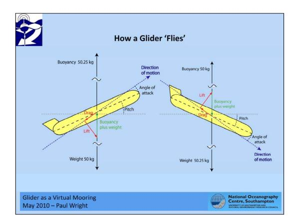
A glider flies by changing buoyancy in the nose by moving +/- 270 cc of oil into/out of a bladder. As it sinks and rises the wings create a lift force that changes a small amount of the vertical motion into horizontal motion. The pitch can be fine tuned by moving the forward battery pack backwards and forewards.
